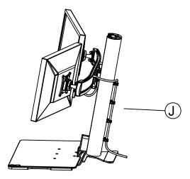
When manage the wires, the tie should be passed through clip to route the wires, adjust the tightness till the last tie is binded. Then adjust the monitor and keyboard holder on the top position, tighten the ties after enough wire length is kept.
