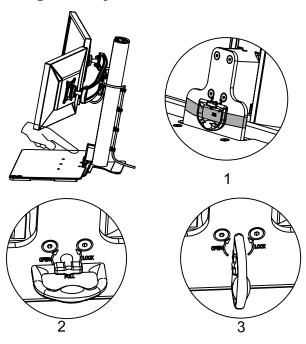
Peel off the protection tape on the handle, pull the handle, and turn 90° in clockwise direction.then freely to adjust up and down. Use reverse operation to lock it.
